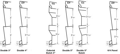
Vertical Board & Batten, Inverted Board & Batten, Half Board & Batten Siding Profiles
